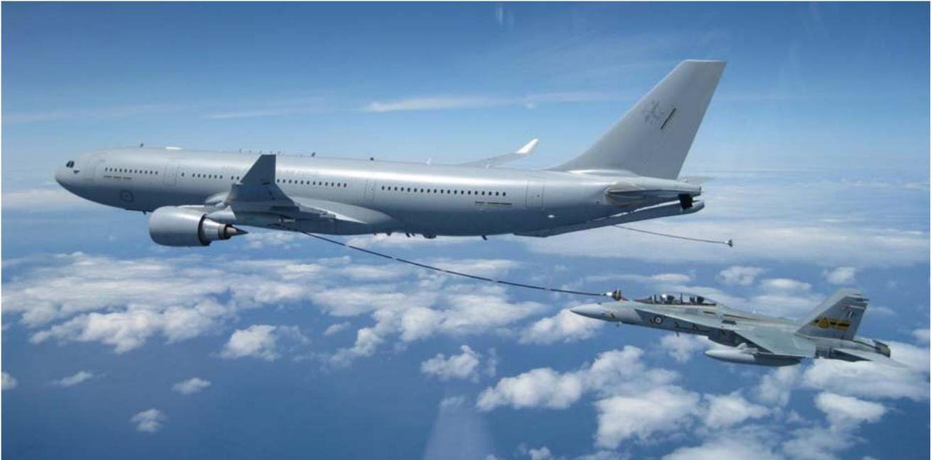
**KC-30A Air to Air Refueling Partial Clearance Testing**
